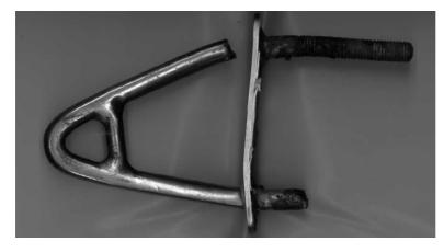
Due to a construction error a piece of screw thread was broken, we were very lucky that the stay hadn't come off the deck! The bolt was tightened too much and wrong positioning meant that the holes of the screw thread had already partly broken off. I have attached a mounting plate below deck as well:
