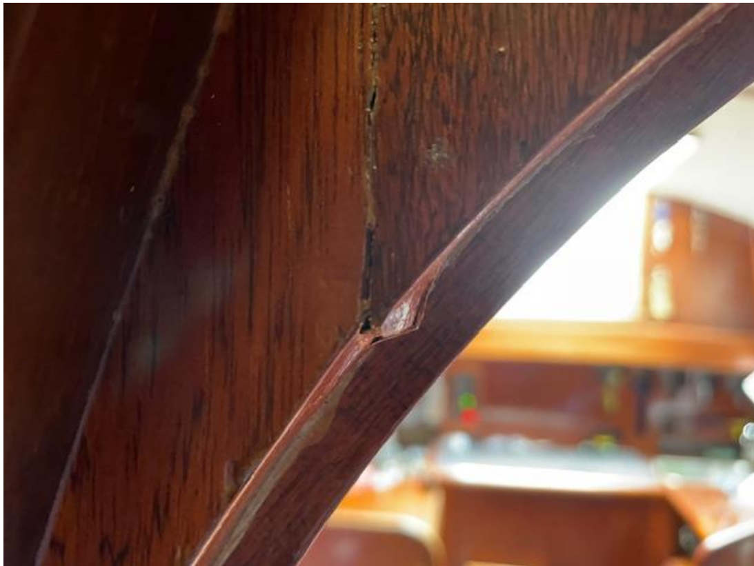
Damage to the starboard side of the main bulkhead due to sagging
