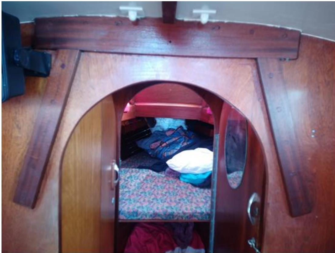
Trintella 1-BN 362-Jadyca-reinforcement bulkhead cabin-side
