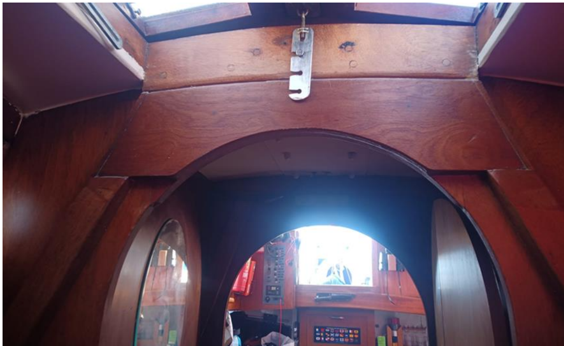
Trintella 1-BN 362-Jadyca-reinforcement bulkhead front side
