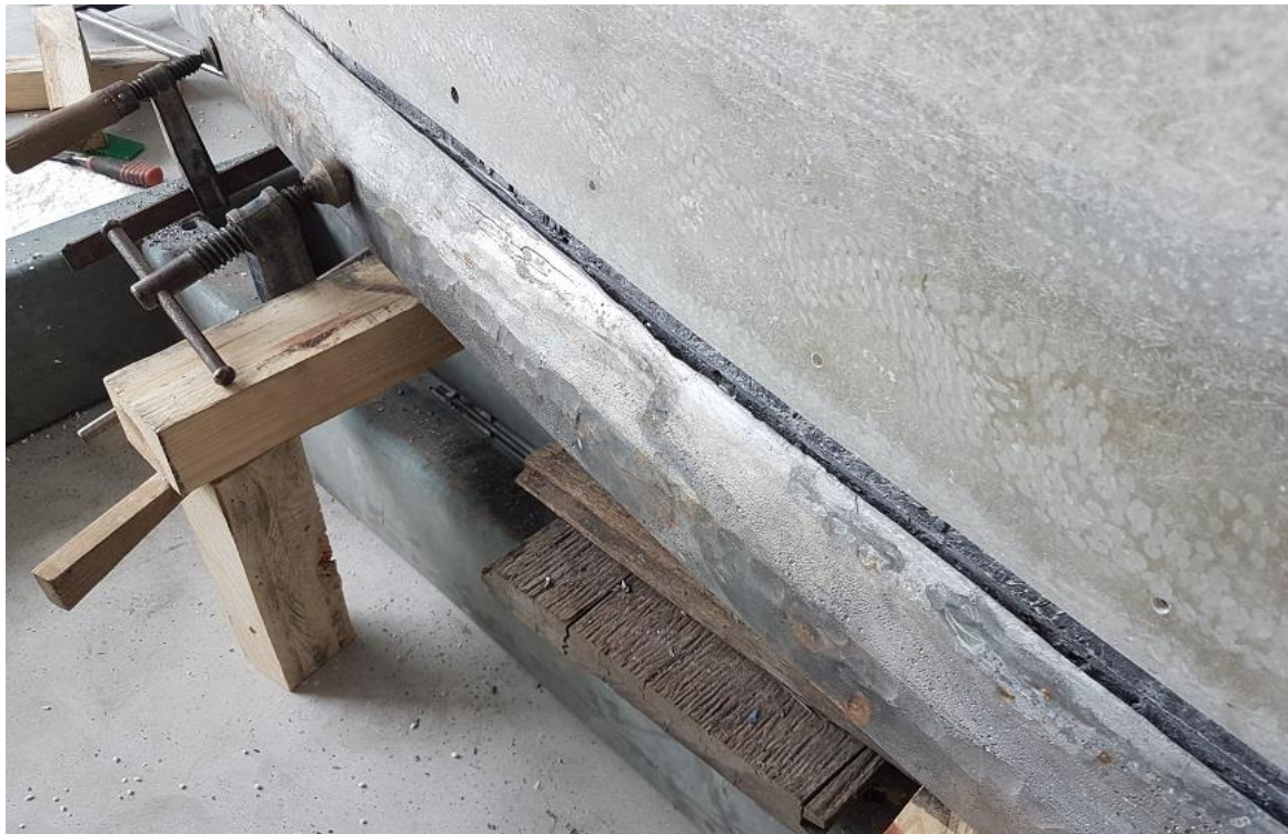
Shaping and gluing the lead strips to both sides of the keel.
