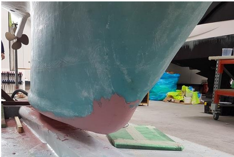
Fairing and glass mat applied. The widened bottom section of the keel is clearly visible.
