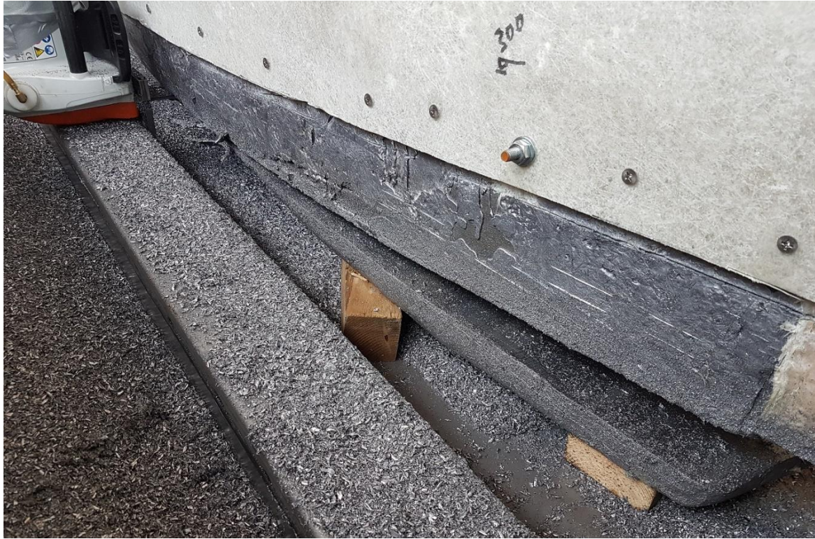
Chainsaw cutting through the keel and the removed lead section.
