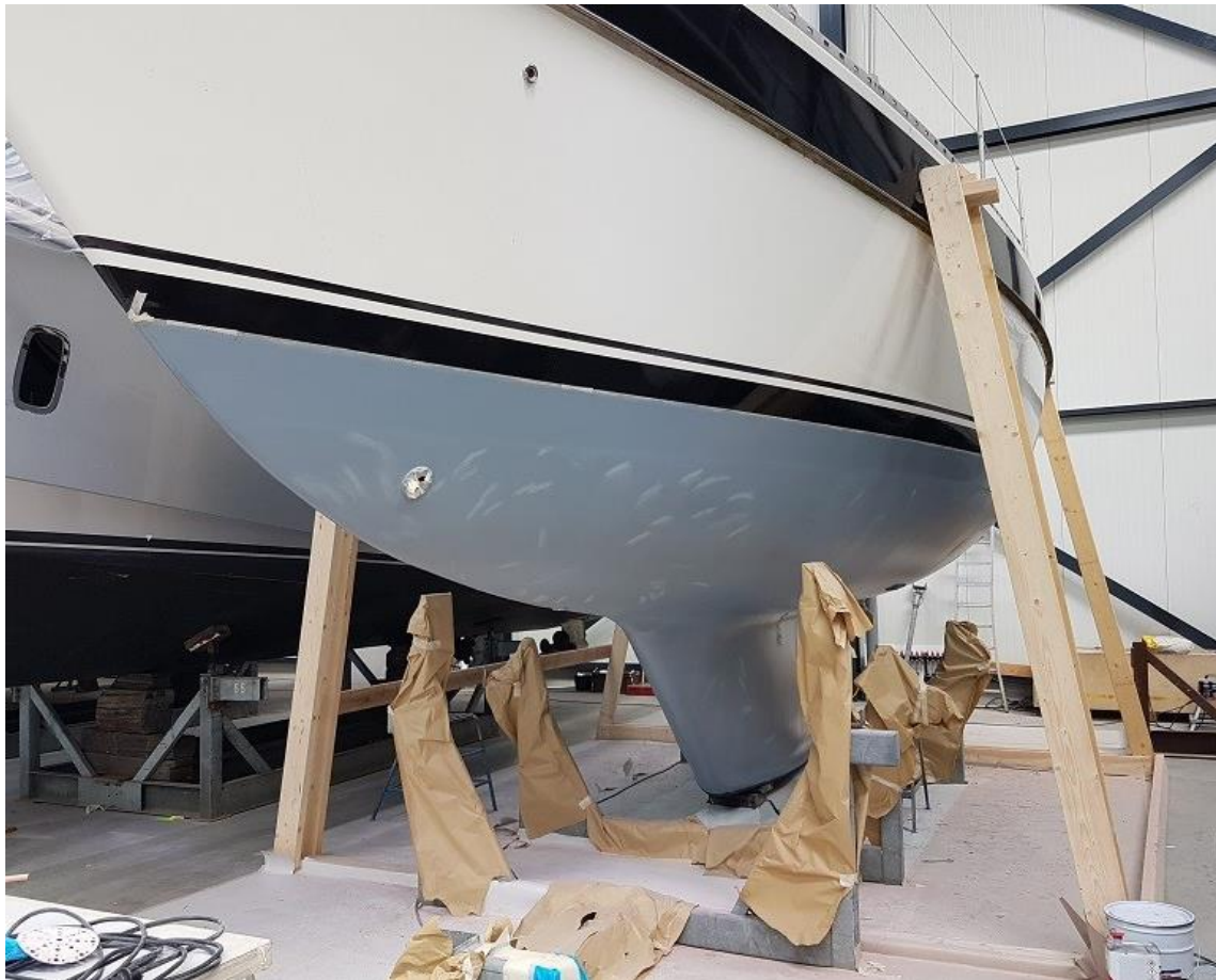
Supported by beams through the windows, allowing full access for painting.
