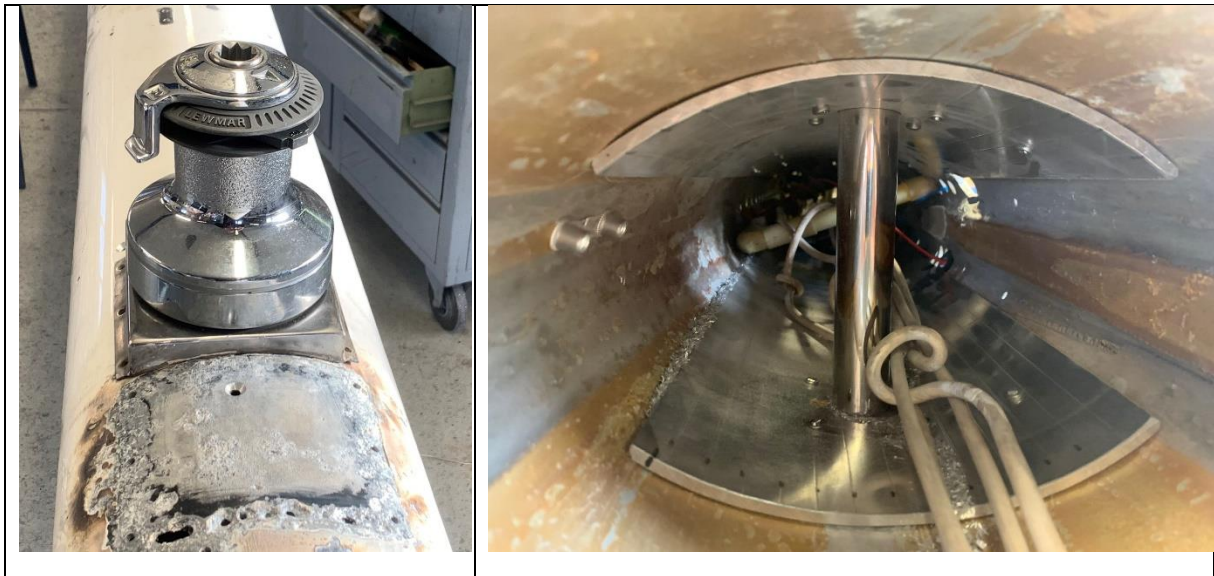
Corrosion under mast winch and repair with insert plates
