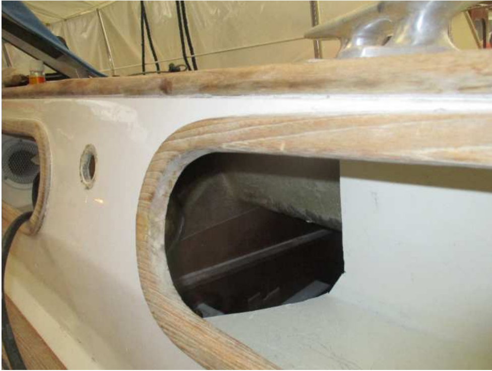
Space for the winch motor
