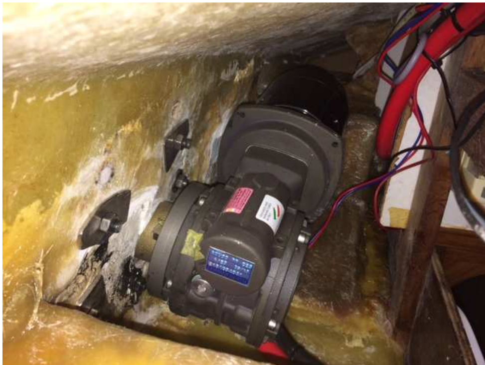
Drive mounted -1. Note the sturdy backing plates.
