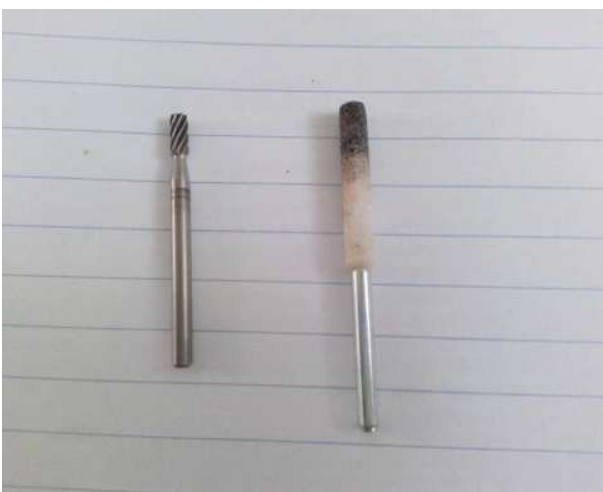
Fig. 13 Dremel router (3.2 mm) and grinding stone (4 mm)
