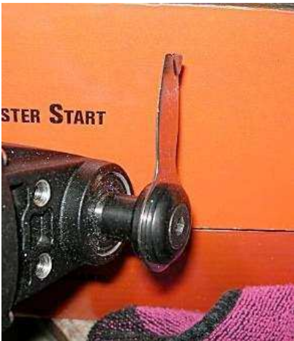
Fig. 5 Fein blade for rubber removal
