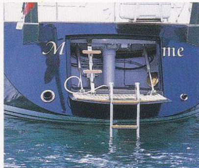
Transom door / swimming platform.
