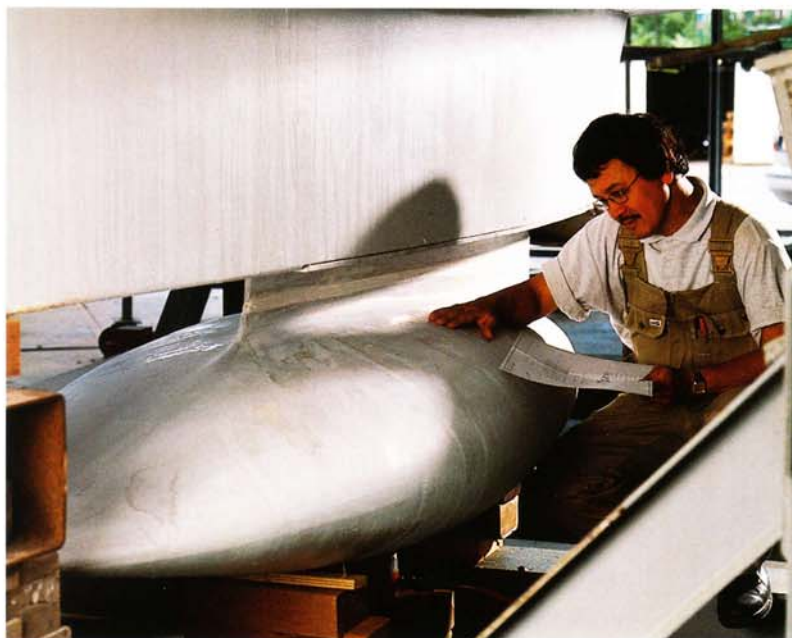
Below: A custom designed hydraulic lifting keel for performance and shallow draft, able to be locked in any position.
