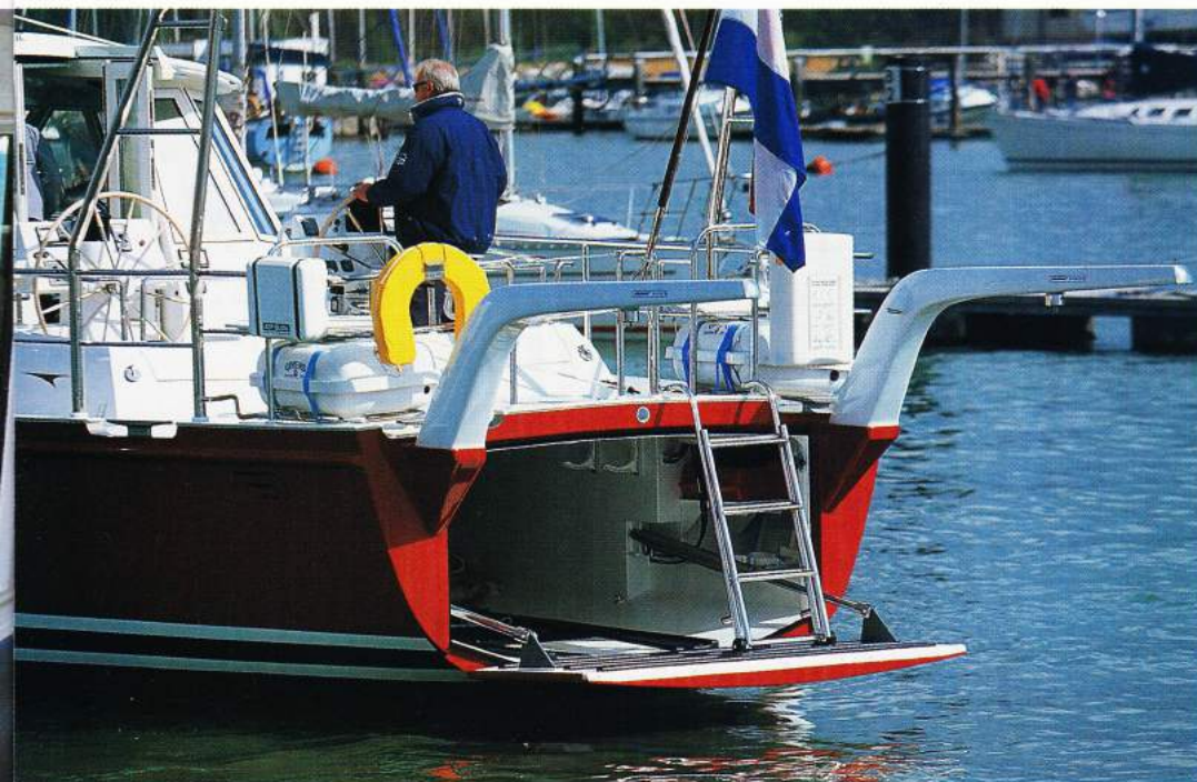
Above: the dinghy garage in the transom is spacious enough to accommodate a GRP dory without even having to remove the outboard
