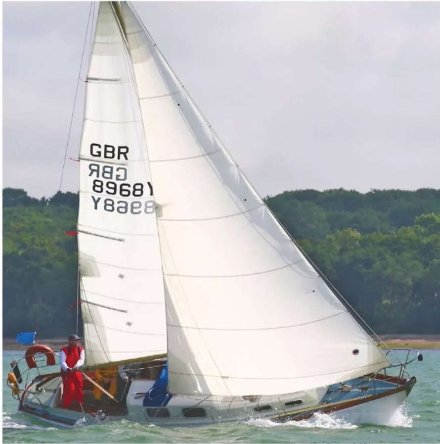
Boats completed in the UK had moulded glassfibre coachroofs
